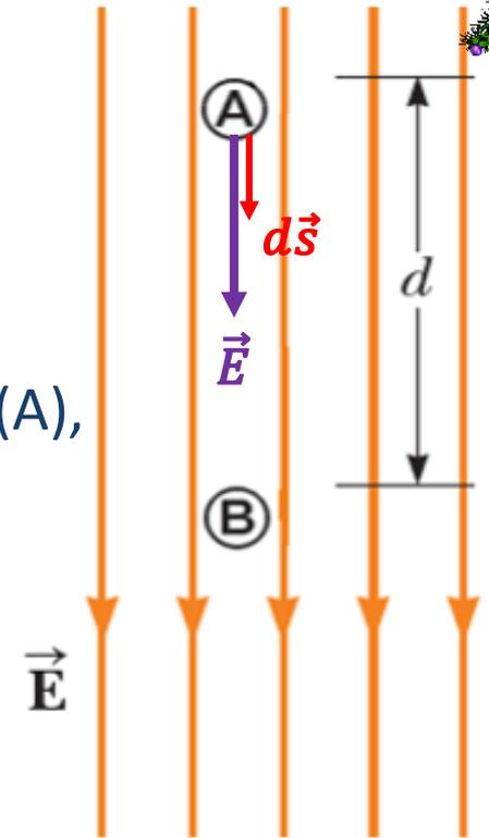
$$\begin{aligned} V_B - V_A &= \Delta V_{A \rightarrow B} \\ &= - \int_A^B \vec{E} \cdot d\vec{s} = - \int_A^B E ds \\ &= -E \int_A^B ds = -Ed \end{aligned}$$
